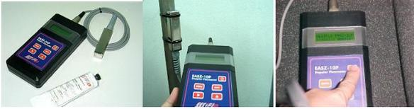
The EESiFlo EASZ-10P Flow Meter measures the velocity of fluids in pipes using a totally non-intrusive principle and gives flow rates and totalized flow in either METRIC or IMPERIAL units
